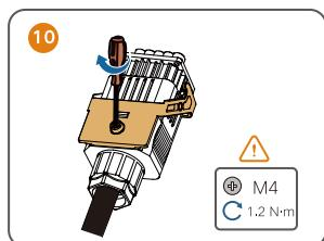
For inverter models  $\geq 15$  kW
