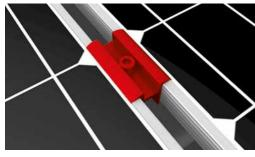
Use two universal module middle clamp OneMid between two modules. Klick the Stance in the notches. Place clamps on the module frames and fix them. Tightening torque 14 Nm.
