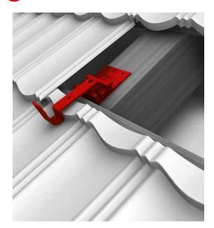
The roof fastener must be mounted with a minimum of 2 stainless steel timber screws on the wooden rafters (at least one screw per row of holes).
