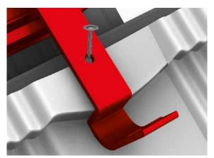
Position the bracket of the roof hook horizontally in order to get into the trough of the tile. To do this, loosen the threaded pin of the bracket. When using the outermost lateral position, the side of the bracket must be flush with the side surface of the base plate.
