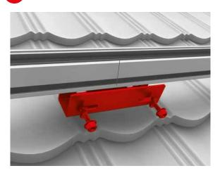
Lay the K2 SingleRail mounting rail butt-jointed and connect it with the help of the rail connector and the 4 hammer-head screws and locking tooth nuts. The rail joint must not be in the area of the roof hook. The connector must be mounted centrally above the joint.
